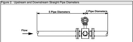
Installations with reduced straight runs from zero to five pipe diameters are possible. In reduced straight pipe run installations, performance can shift as much as 2 percent of rate. Reported flow rates will still be highly repeatable.
