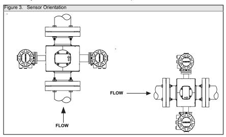
The electrodes in the Rosemount 8705 sensor are properly orientated when the two measurement electrodes are in the 3 and 9 o'clock positions, as shown on the right of Figure 3.
