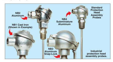
The  $\frac{1}{2}$  NPT mounting thread allows  $\frac{1}{4}$ " OD industrial protection head assemblies to be put directly into OMEGA® thermowells whose bore is 0.260" without having to use any additional hardware. In this case, the probe length must be the same as the element (stem) length of the desired thermowell.
